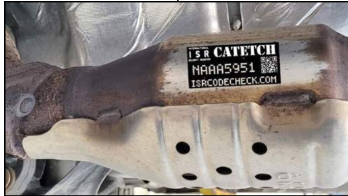
An anti-theft ID on an older catalytic converter. (mastergard.com)
